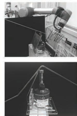
Fig. 11.1. Angle bending experiment
